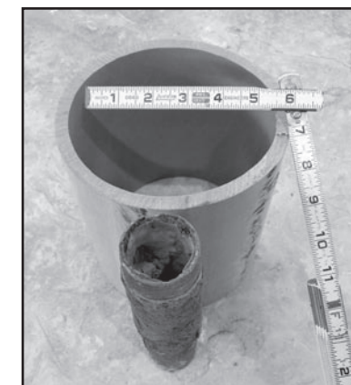
Cross-section of new 6" HDPE pipe installed at Cove Lane, compared to cross-section of old 1 1/2" pipe. Note accumulation of mineral and iron deposits inside old galvanized pipe.
